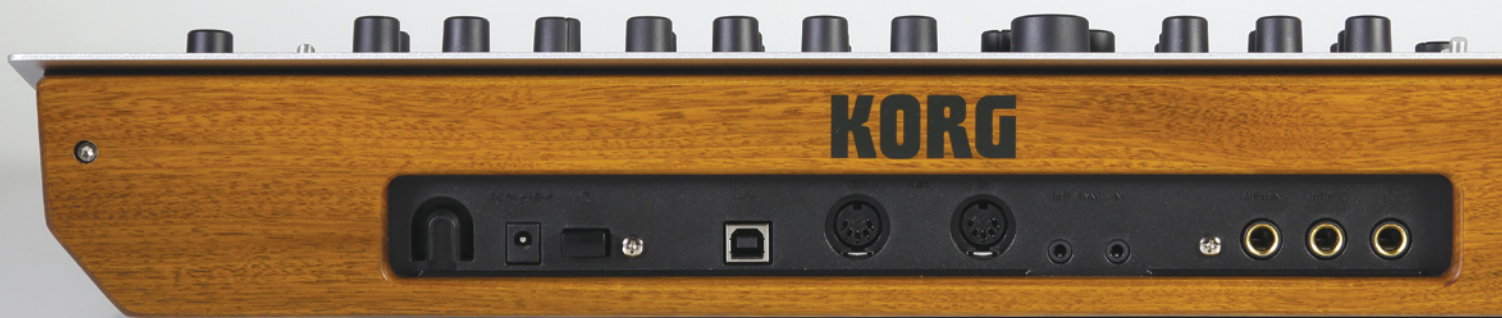
The Minilogue's (surprisingly few) sockets are all to be found recessed into the wooden rear panel.
